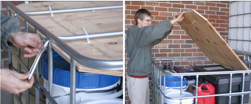
Figure 5 – Remove Plywood Cover from Cage 2
