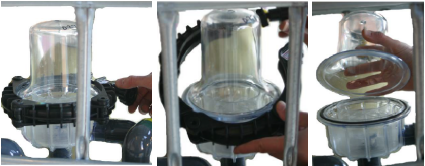
Figure 26 – Remove the Chlorinator Cover
