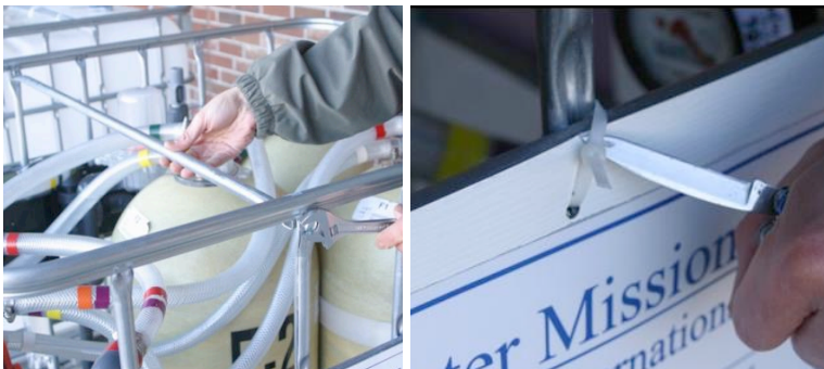
Figure 7 – Reattach Bars and Remove Protective Sheet
