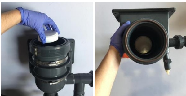
Figure 11 - Add Chlorine Tablets
