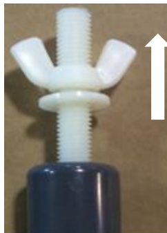
Figure 15 - Threaded Rod Pulled Out and Flush with Wing Nut
