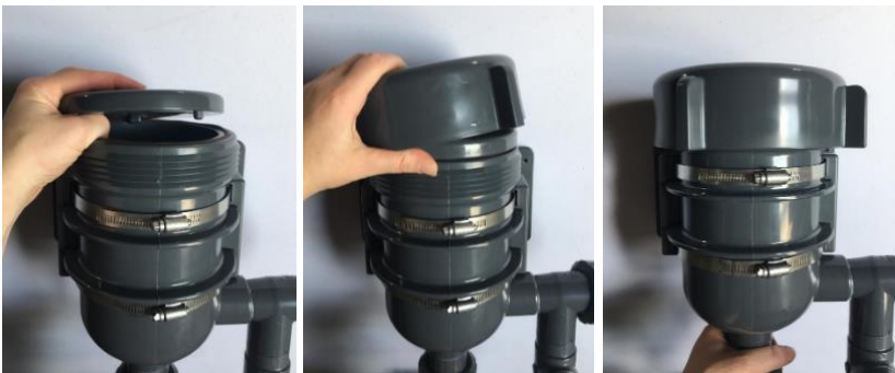
Figure 13 - Replace the Cover
